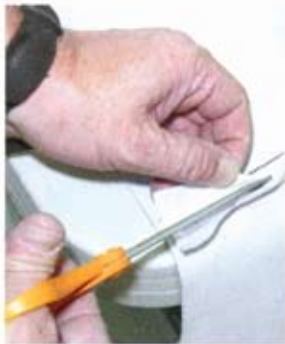
4 Before installation, Richard suggests carefully cutting the headliner sheaths just enough to allow flexibility at the sides. Don't cut too much.
