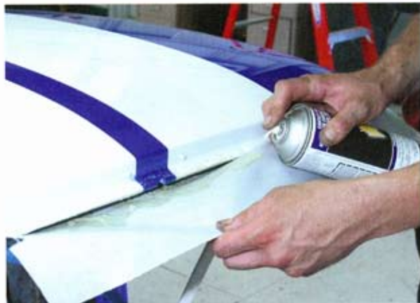
17 Headliner is glued and secured in front, making sure all wrinkles are gone.
