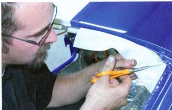
18 Richard carefully cuts the headliner to create smooth, flexible corners when securing the headliner.
