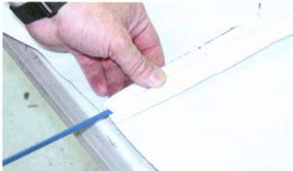
3 Headliner bow location is very important. Ford had its own color-coding system for headliner bows. Although Richard has come up with his own color coding system based on the way these bows came out, here's what you can expect to find from an original car. Colors may vary from generation to generation and plant to plant: Front: natural or purple (shortest bow); second bow: green (next longest bow); third bow: pink (next longest bow); fourth bow (hardtop only, longest bow): natural or plain.
