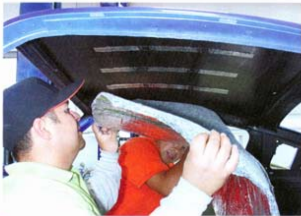
2 Quiet Ride Solutions installed sound deadening in Reclaim, which will make a tremendous difference in ride quiet. It's affordable and very effective.
